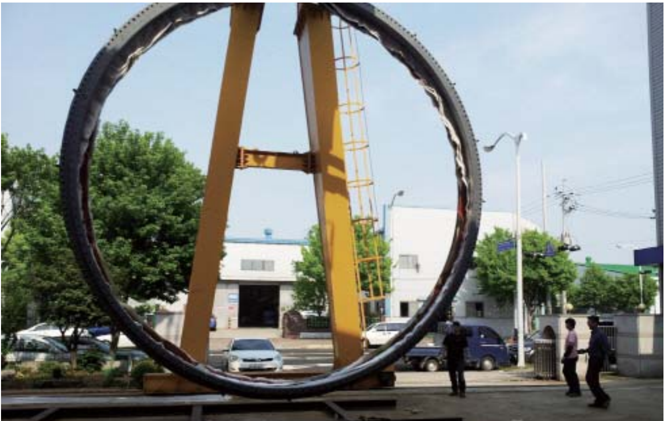
8000mm diameter integrally flanged type fabric expansion joint
