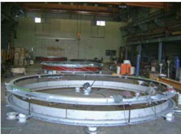
Integrally flanged type expansion joints with metal frame and baffle before fabrication of flexible elements
