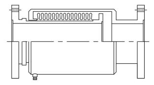
When a pipeline expands, expansion joint compresses, but it stretches the bellows. Bellows remains stable due to external pressure
