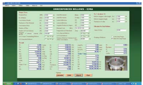
Kurbo's bellows design software developed to cater to the design and analysis of the expandable metal bellows
