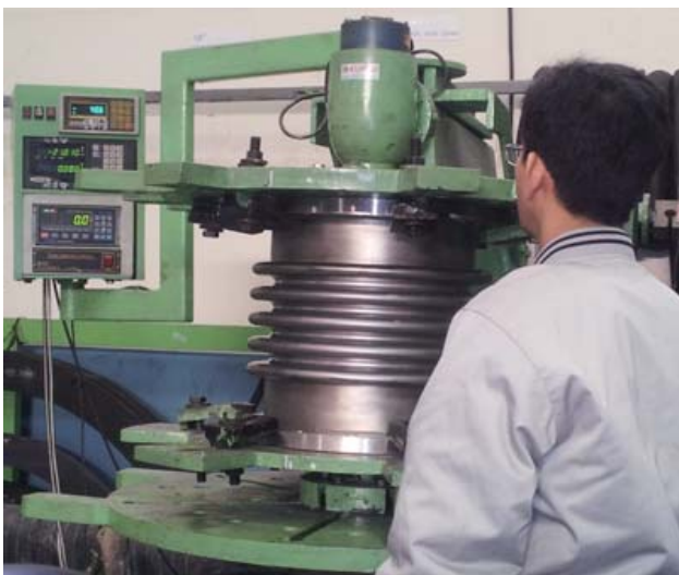
Verifying bellows design through movement/spring rate testing
