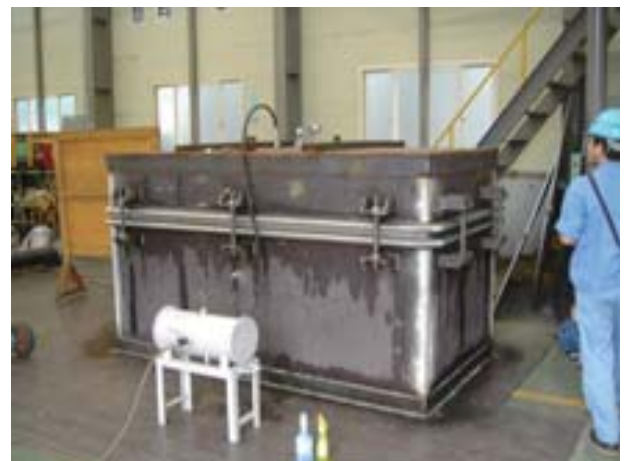
Kurbo's inspector performing hydrostatic test
