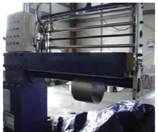
Longitudinal seam welding after rolling tube
