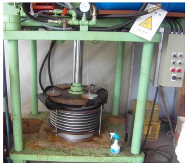
Kurbo's 600mm diameter single expansion joint being hydrotested before painting and packaging
