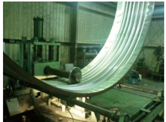
Mechanical roll forming of bellows
