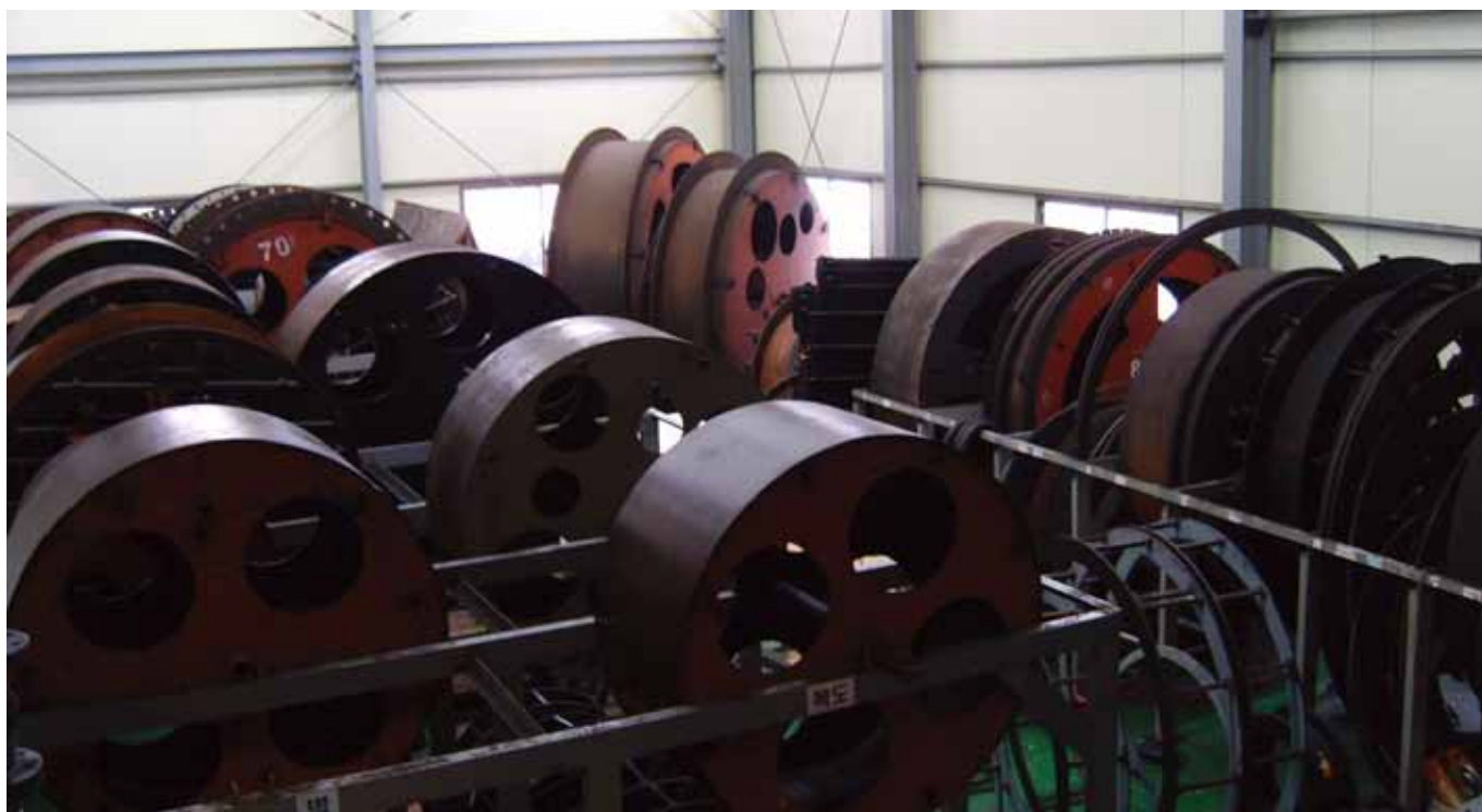
About 270 units of mandrels are ready for immediate production when ordered. Various sizes and shapes including concentric/eccentric, elbow and rectangular etc are available. The largest size of mandrel we have is 3600mm diameter.
