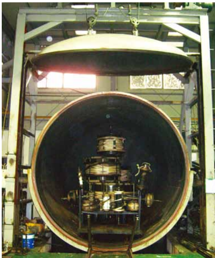
After the product with uncured rubber has been built on the mandrel, it is placed in the autoclave for curing. Pressurized steam curing imparts design characteristics of finished product.
