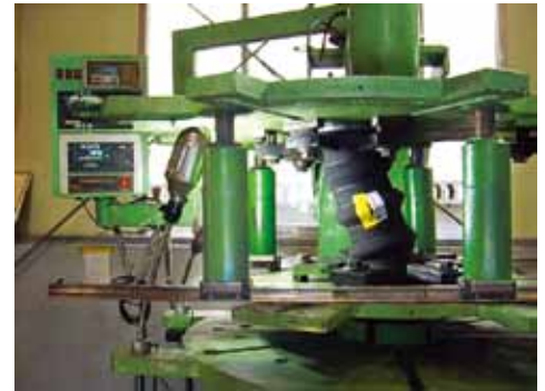
Shown above is 100mm lateral deflection of WinFlex Type 23UG, DN100 x 350mm
