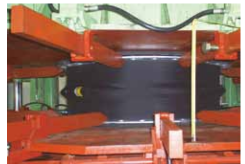
Combined deformation test in axial and lateral direction. Available sizes for flex testing are up to DN1650.
