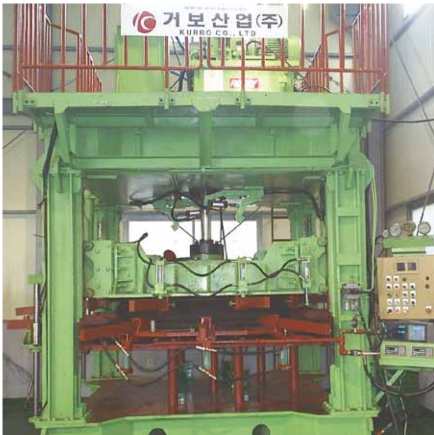
Combined deformation test in axial and lateral direction. Available sizes for flex testing are up to DN1650.
