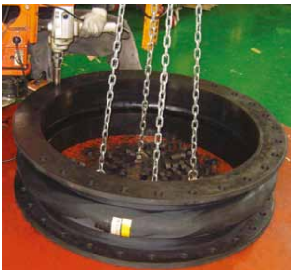
After cure, the flange holes are drilled clean with hollow and sharp drill cutter.
