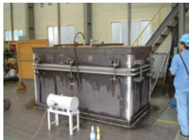
Kurbo's inspector performing hydrostatic test
